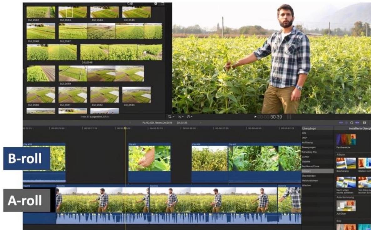
Figure 27. Arrangement of A- and B-roll in the editing program. Images of the B-roll are used to cover cuts in the A-roll and to visually support what has been commented on in A-roll. (source: Deliverable 4.3-PLAID)
